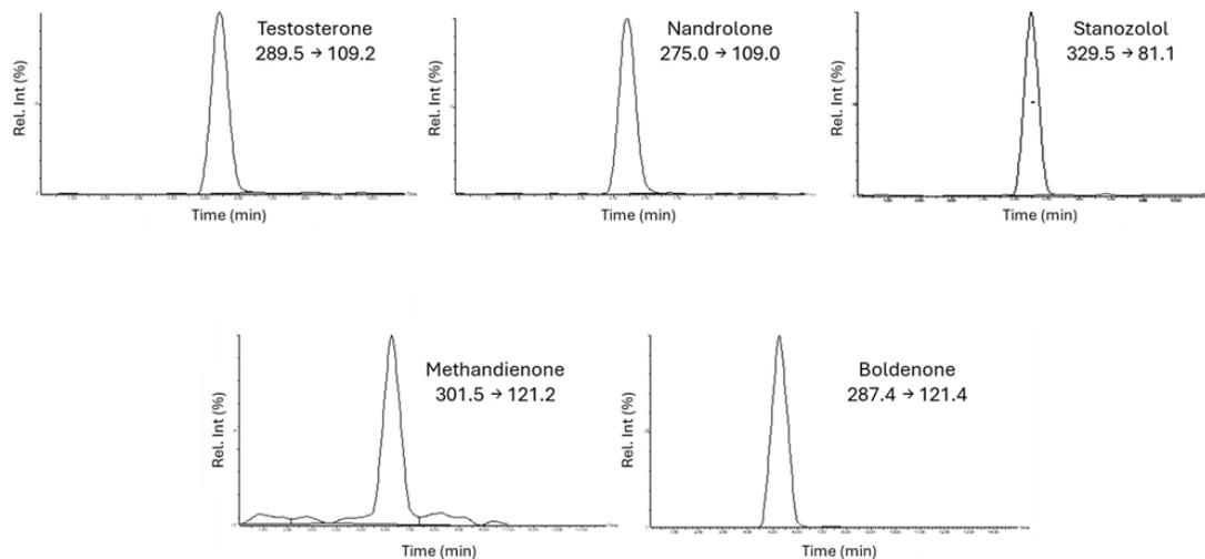
**Figure 3** | Representative HPLC-MS/MS MRM chromatograms of a blood VAMS sample fortified with the analytes, showing clear peak separation and lack of interference.
